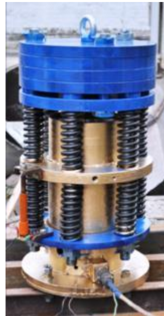
Vibro-hammer based on coaxial-line engine with permanent magnets
