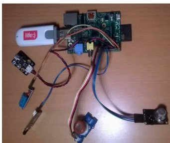
The model of WSN node for the remote sensor-assisted temperature and humidity monitoring
