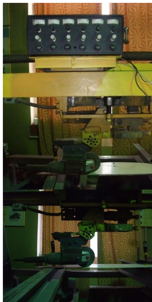
The working equipment fixed on the stand for the surfaces cleaning force measurement
