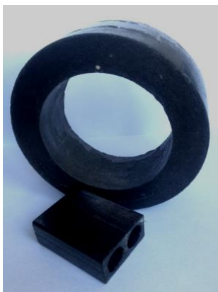
Component parts of the micro-injector MK 10-1 (rotor 90 × 60 × 34, plate)
