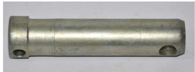
Bush and finger with a reinforced coating
